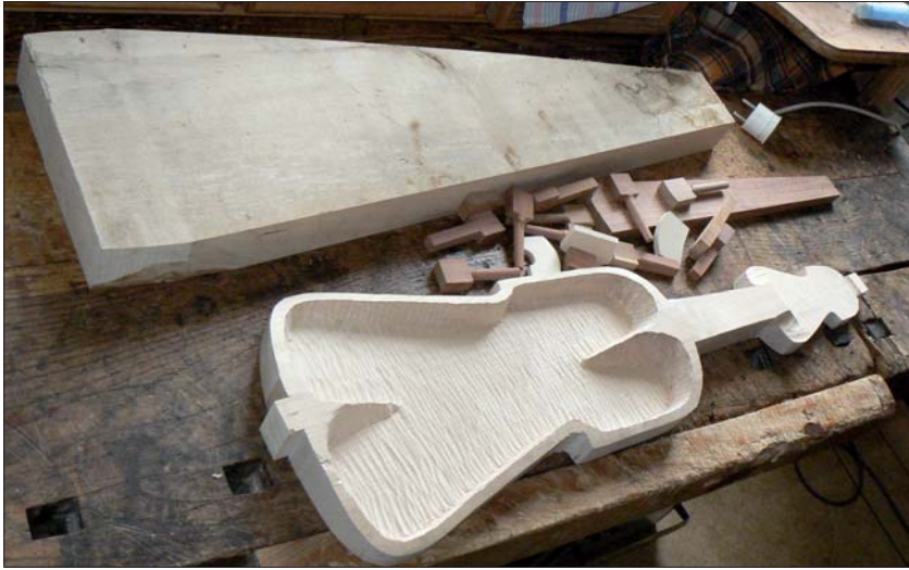
Fig. 4: Detail of the instrument's corpus before it was closed by the top plate. In the upper part, there is material for the construction of another instrument. Photo by Jiří Höhn 2013. NULK Archives.
